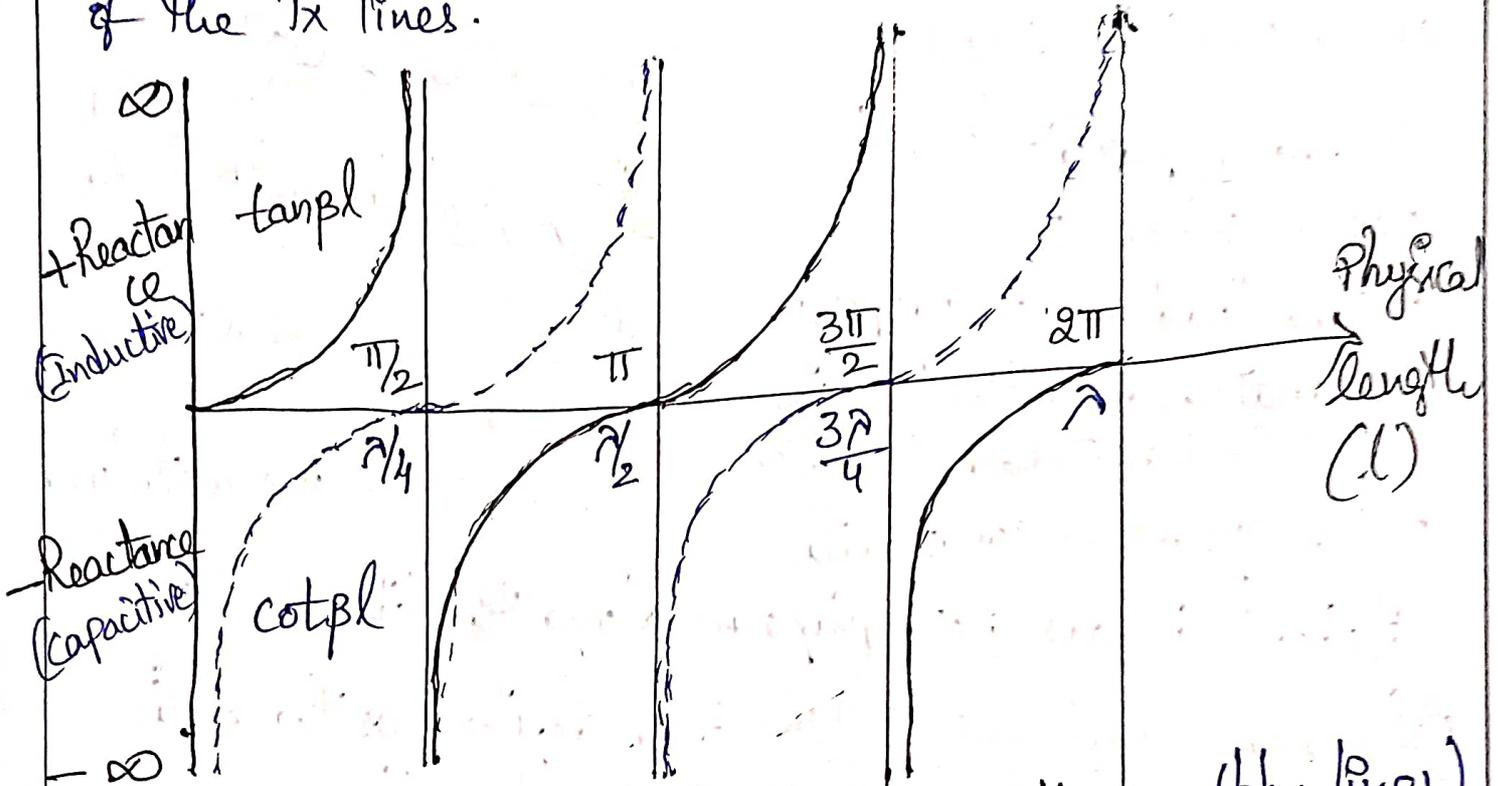
fig: variations of the input impedance with  $Z_{oc}$  (blue lines) &  $Z_{sc}$  (black lines).
