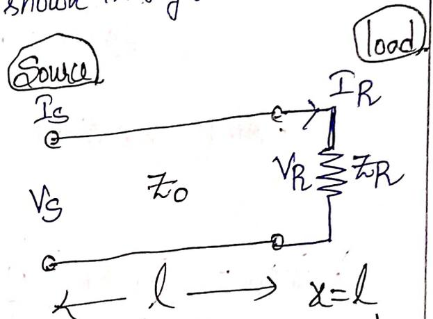
fig: Tx line with load from sending end
