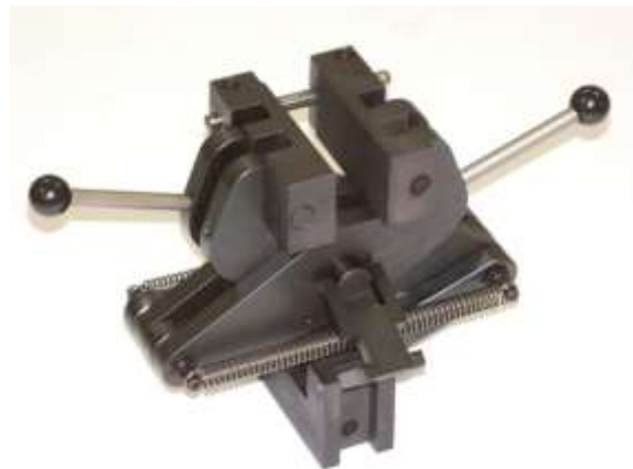
Fixture(Pincer grip for material testing in tensile tests.)
